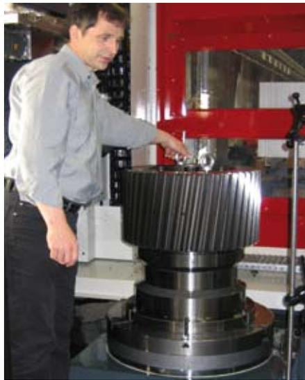
*Königdorn® clamping tool Type E with a clamping diameter of 360 mm. During gear grinding processing the workpiece, a gear with an outer diameter of 1,000 mm and a weight of 1.2 t, reaches a run-out accuracy of  $\leq 0.01$  mm.*
